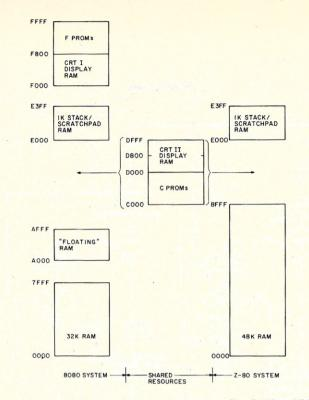
Fig. 2. The memory maps of the two processors. The RAM and ROM memory segments of the shared resources can appear in the address space of either processor, depending on the position of the bus switch.
